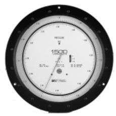
Series 1500 Differential Pressure Gauges have capsule-type pressure elements. High differential pressure is applied to the capsule; low pressure to the case. Available in 22 standard ranges, they combine aneroid convenience with liquid-column accuracy. And they are rugged enough to maintain their high accuracy in test and process applications.
